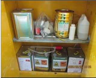
Photo of non-conformity NC no safety labels posted on chemical containers.JPG
