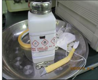
Photo of non-conformity NC chemicals safety label was incomplete.JPG
