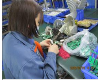
Photo of non-conformity NC the factory did not provide dustproof masks for soldering worker.JPG
